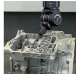
REVO 5-axis measurement system
