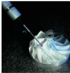
High speed SP25 scanning probe
